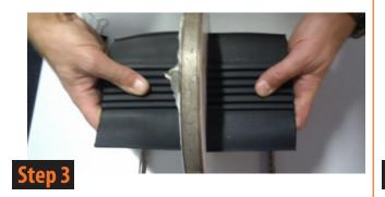
Heat the Seal ends on the Heatpad for 30 seconds at 220°.
