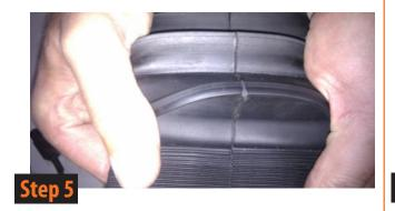
After the weld has cooled down (approx 2-3 minutes) test the weld by applying some force to seals at the weld.
